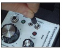
2. Plug the white connector cable (B) into the jack labeled Pads. Make sure the plug goes in all the way and is firmly seated. Remove a pair of pads from the sealed envelope. (When not in use, store them in the sealed envelope to prevent them from drying out.) You will find that the connector cable splits into two at one end. Push each pin into an electrode connector.
