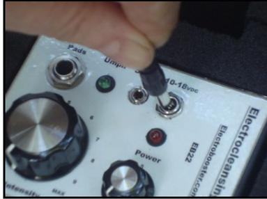
2. **Plug the white connector cable (B)** into the jack labeled Pads. Make sure the plug goes in all the way and is firmly seated. Remove a pair of pads from the sealed envelope. (When not in use, store them in the sealed envelope to prevent them from drying out.) You will find that the connector cable splits into two at one end. Push each pin into an electrode connector.
