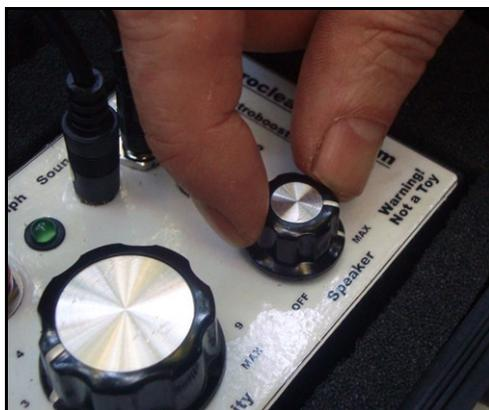
6. Gently turn the Intensity or volume knob until you can hear and feel the electricity (typically between 1 and 3). Do this slowly and with caution until you find a comfortable level. The green Umph light will flash, indicating the strength and intensity.
