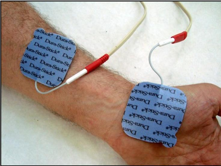
*Note: After the pads have been used many times, you may need to rub several drops of water into the pads to revive the stickiness. Also, if the pads are too old or well used, they may not be reliable electrical conductors. Replace with new ones.*
